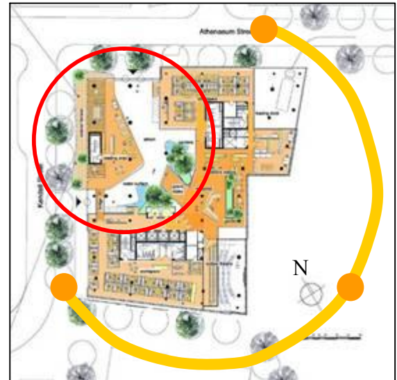
Figure 5: Orientation: The atrium (red circle) on the Northern side serves as a heat loss buffer. The orange semi circle represents the sun's path
